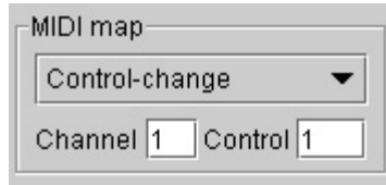
Fig. 2-4-4: The MIDI map section of a sensor window with the sensor value mapped to a control-change number 1 message on MIDI channel number 1.
