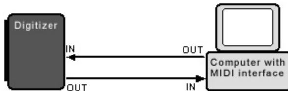
Fig. 1-1: Stand alone mode basic MIDI signal path between the Digitizer and computer.
