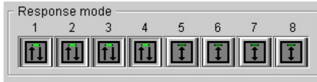
Fig. 2-5-2: The response mode section of the actuators window with outputs 1-4 set to toggle mode.
