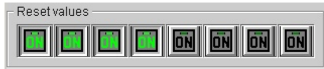
Fig. 2-5-3: The reset values section of the actuators window with all outputs set to turn on after a Digitizer reset.
