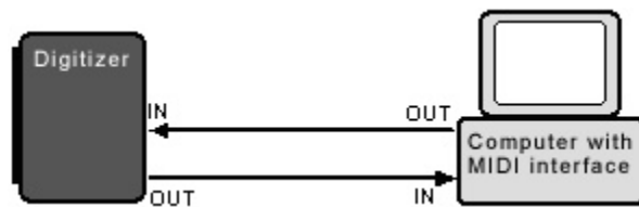
Stand alone mode basic MIDI signal path between the Digitizer or miniDig and computer.
